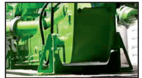
Boom Section Feet prevents from scratch and corrosion
